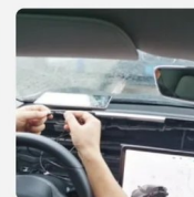
15. Connect the dashboard trim panel with the product installed to the power supply
