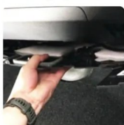
8. Pull out the bottom flap of the glove box
