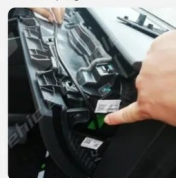
13. After connecting A and A1, put it through the position pointed out by the finger and fix the power cord with adhesive tape, which cannot block the position of the snap
