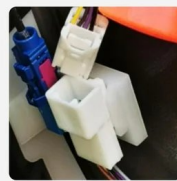
10. After unplugging the original power connector B, connect the female connector to B1 and the male connector to B2
