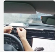
15. Connect the dashboard trim panel with the product installed to the power supply
