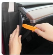
1. Removal of the instrument panel (left side)
