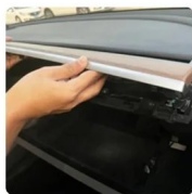
4. Remove the dashboard trim panel
