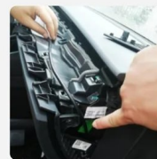
14. After connecting D and D1, put it through the position pointed out by the finger and fix the power cord with adhesive tape, which cannot block the position of the snap
