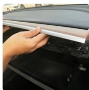
4. Remove the dashboard trim panel
