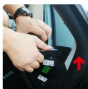
3. Raise the instrument panel vertically upward from the left and right sides
