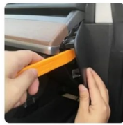
2. Removal of the dashboard (right side)
