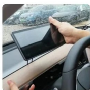
5. Plug the power cord into the 37th and 39th holes counting from left to right, blind holes do not count in the count. Insert the machine into the dashboard trim panel by aligning the holes
