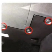
7. Pry open the trim panel clips at the bottom of the glove box at the passenger side
