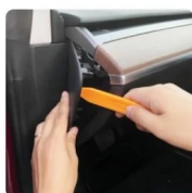
1. Removal of the instrument panel (left side)
