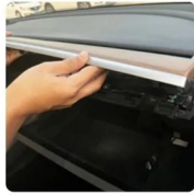
4. Remove the dashboard trim panel
